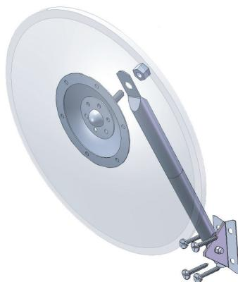
Attach arm to swivel ball on hub.
