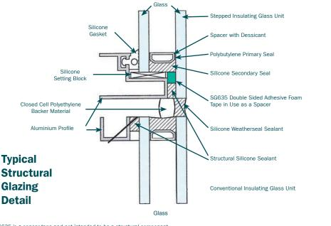
SG635 is a spacer tape and not intended to be a structural component
