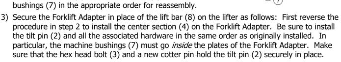
Note: Clean hardware and replace any worn-out hardware, as necessary. In particular, **the cotter pin must be replaced**, as it is only intended for one-time use (see REPLACEMENT PARTS LIST).
