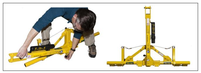
Attach the hoisting equipment hook to the lift spool as shown.
