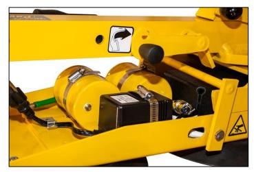
Then disengage the tilt latch and raise the <u>lift bar</u> to a vertical orientation, as shown.
