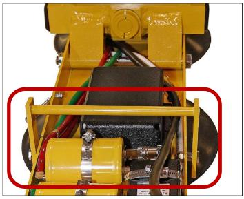
Lower the <u>lift bar</u> to make sure the tilt latch engages correctly, as shown.
