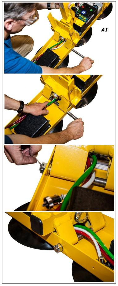
5) Install the <u>tilt latch bar</u> on the <u>pad channel</u> using the hardware supplied, as shown.
