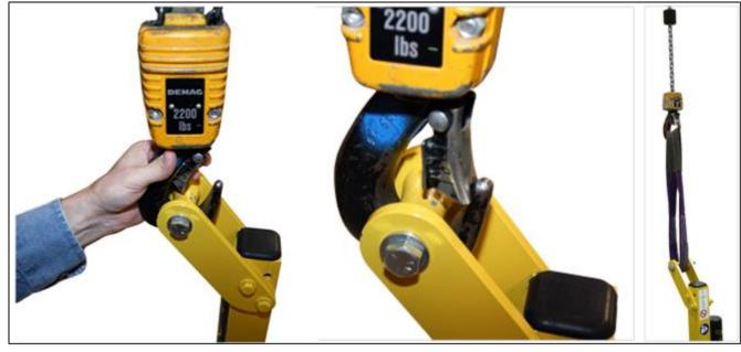
Make sure hoisting equipment hook is fitted with restraining latch to prevent lift spool from slipping off under any circumstances.
