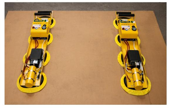
3) Use the hoisting equipment to position the <u>lift frame</u> between the rails of the <u>pad channels</u>, as shown.
