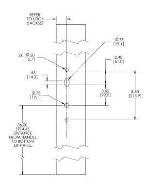
FIG. 8 SENTRY HINGED PATIO DOOR HANDLE SET, PASSIVE ASSEMBLY
