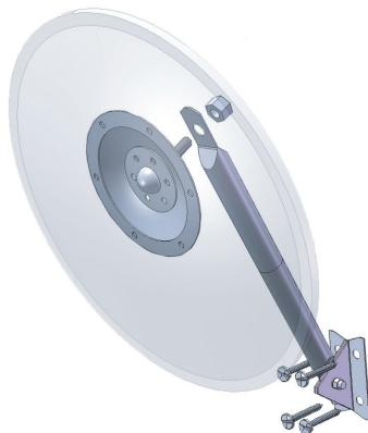
Attach arm to swivel ball on hub.
