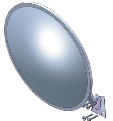
Back off 1 or 2 screws on hub, 1/2 turn only. Adjust angle of mirror, retighten hub screws.
