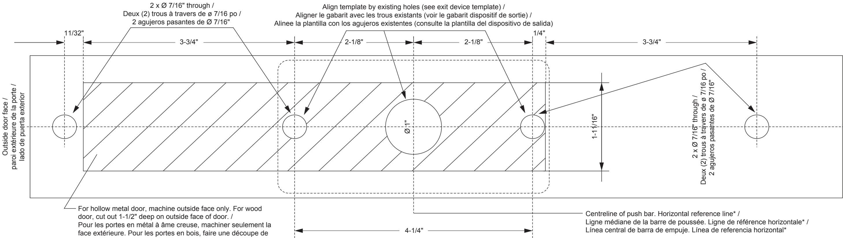
For hollow metal door, machine outside face only. For wood door, cut out 1-1/2" deep on outside face of door. /
