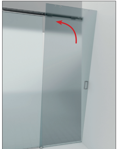
20- Bring the door inside the shower stall. Place the 3 mm gasket on the trolleys. Slide the door first into the floor track, then straighten it and secure it to the trolleys by repositioning the octagonal studs and screwing them on. Do not tighten all the way.
