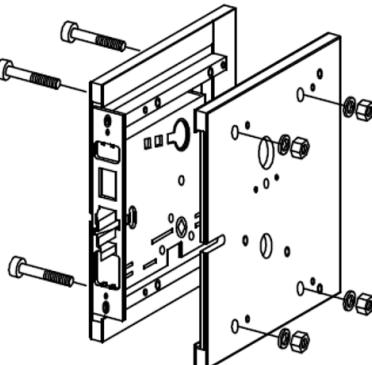
Split clamp plates by removing screws.
