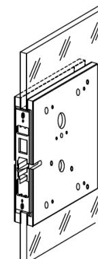
Before finally tightening, test install the face plate and the cover plates to ensure alignment with glass and each other.
