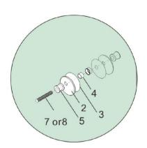
Install the handles onto the collars, making sure the washers are properly aligned
