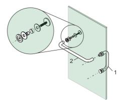
Install the set screws and tighten with the Allen key to finish the installation.
