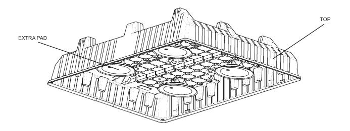
Attach rubber straps to secure top of case to bottom.
