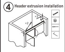
Finish installing the header by screwing in the mounting screws and assembly screws.
