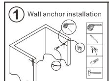
Mark the location of the header brackets and ensure they are level to avoid problems after installation. Drill the holes at a 30° on both sides and insert the bracket anchors.
