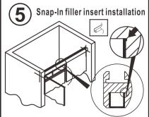
Measure the open channel space above the door. Cut and install the Snap-In filler insert into the header extrusion
