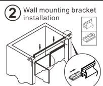
Slide the brackets into the header extrusion. For 12mm glass, simply press the extrusion down directly onto the fixed glass panel. For 10mm glass, see step 3.
