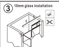
Cut the clear gasket to the desired length and install tightly onto the fixed glass panel then press the extrusion onto the panel.
