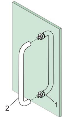
Install the set screws and tighten with the Allen key to finish the installation.
